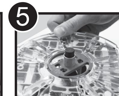
**5** After lowering the Base Plate so it is in contact with the centering pin, rotate the Base Plate over the router's threaded screw holes until the correct alignment is found.
