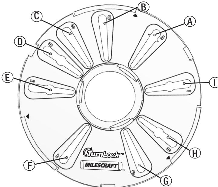
In some instances shown above, NOT ALL holes in router's base will match the mounting pattern. Only two diagonal holes matched to a router's base are required (as a minimum) for proper installation and operation. You may decide to modify an existing slot or add hole(s) to better suit your router. The screws supplied may not fit your router. If you supply your own screws, DO NOT use "counter sink head styles".
