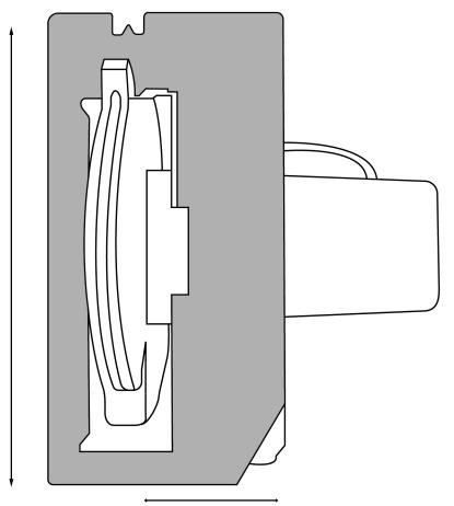
3-5/8" to 5-3/8" Edge of Saw Base to Inside Face of Blade
