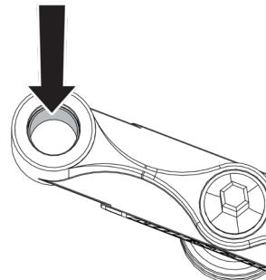
From top, push lip of bushing using flat screw driver or similar item to remove.
