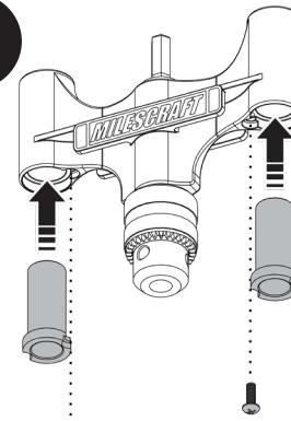
Insert new bushings and reinsert screws.
