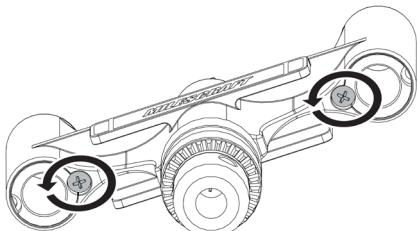
Remove the two screws in the Guide Head.
