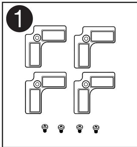
The DrillMatePRO™ includes four non-slip pads and four M5 screws.
