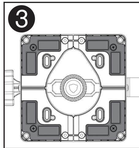
All four pads will provide the largest possible non-slip surface for the DrillMatePRO™.
