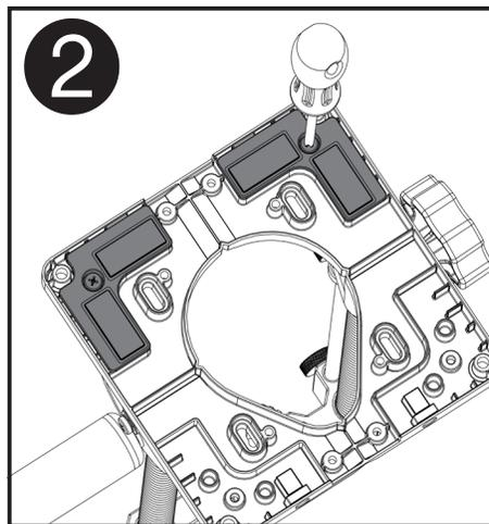
Place the four pads in the corners at the bottom of the base plate and secure them with the four screws.
